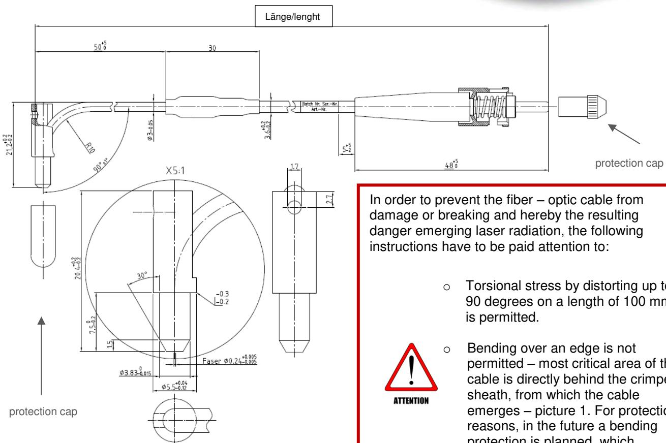
In order to prevent the fiber – optic cable from damage or breaking and hereby the resulting danger emerging laser radiation, the following instructions have to be paid attention to:
