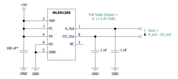
\* if the supply voltage is disturbed by EMI it can be useful to place a second capacitor (100pF ceramic) parallel to the 100nF capacitor.
