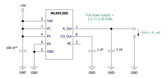
\* if the supply voltage is disturbed by EMI it can be useful to place a second capacitor (100pF ceramic) parallel to the 100nF capacitor.
