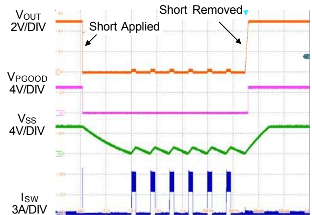
Figure 3. Short-Circuit Protection and Recovery
