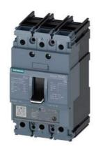
circuit breaker 3VA5 UL frame 125 breaking capacity class S 25kA @ 480 V 3-pole, line protection TM230, FTAM, In=90A overload protection Ir=90A fixed short-circuit protection Ii=5...10 x In nut keeper kit on both sides
