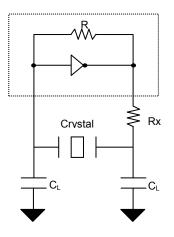
$C_L = 2^*(C_P - C_S), \\ Where C_P = Load capacitance of crystal \\ C_S = Stray capacitance due to C_{IN,} PCB, Trace etc.$
