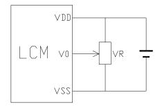
V<sub>DD~</sub>V<sub>0</sub>: LCD Driving voltage
