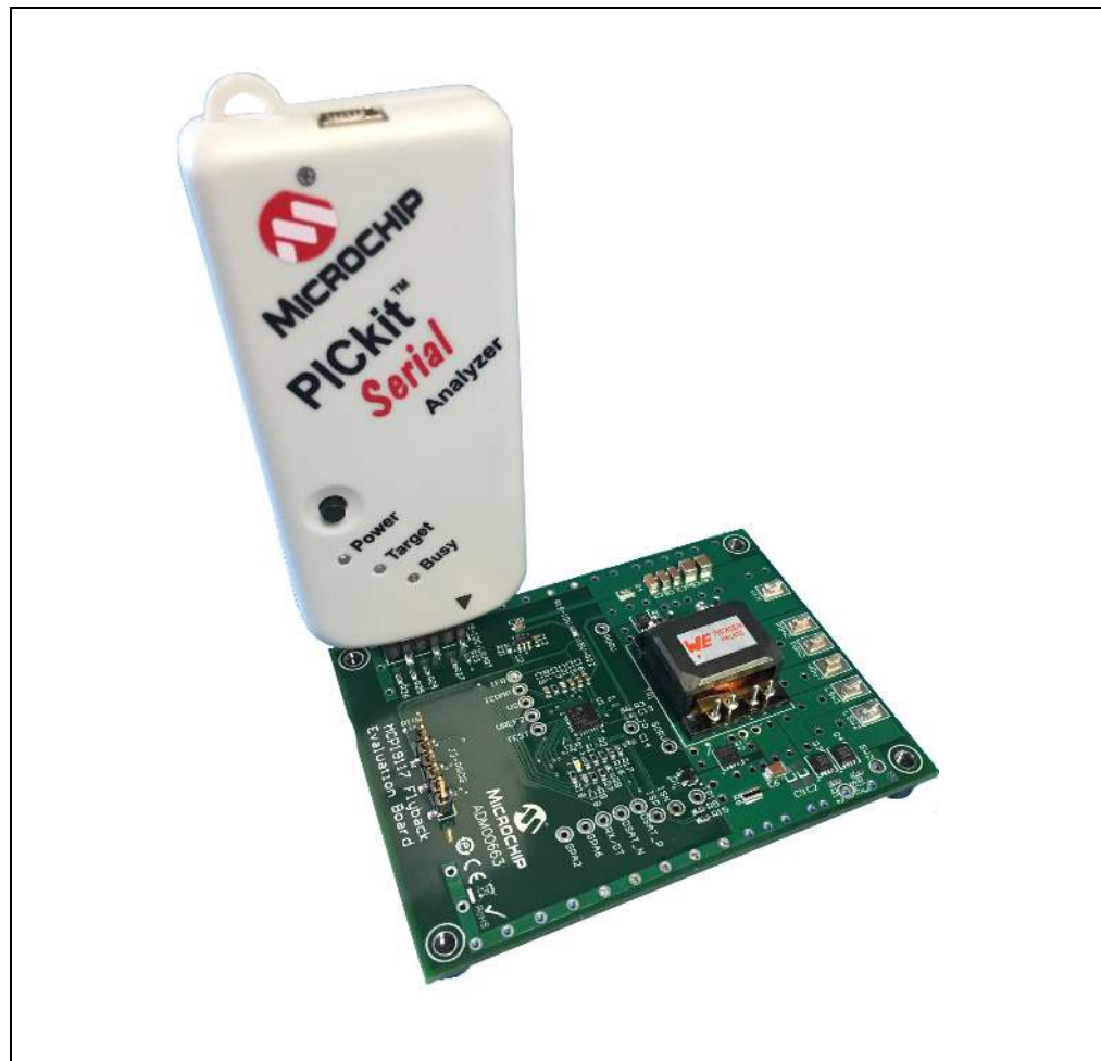
FIGURE 3-1: PICkit Serial Analyzer Connection to the Board.
