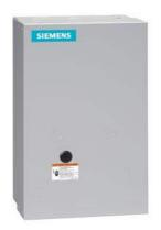
2-speed 3-phase motor starter Size 3 Two separate windings Constant or variable torque Solid-state overload relays Low SPD OLR range 25-100A High SPD OLR range 25-100A 110V 50HZ / 120V 60HZ coil Enclosure NEMA type 1 Indoor general purpose use
