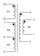
N2 denotes two windings connected in parallel. Terminals 1+2 and 4+5 must be tied as solder bridging is allowed.
