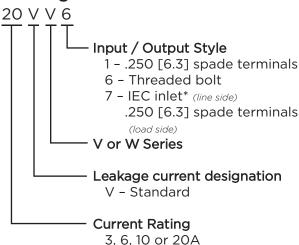
\*IEC 60320-1 C20 inlet mates with C19 connector
