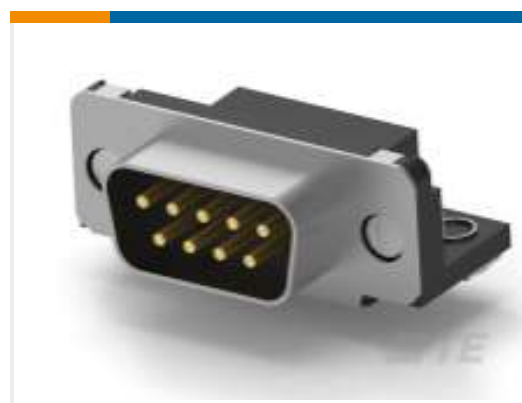
TE Part #5747250-4 D-Sub Plug Assembly: Standard, Right Angle, Shell Size 1, 2.74mm
