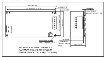
**Note**: This open frame power supply should preferably be mounted horizontally on 4 metal stand-offs having diameter not more than 6mm and height not less than 5mm
