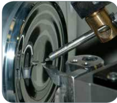
Rotation-symmetric multiple aspherical surface, aluminium.
