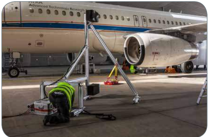
The DLR Institute of Aerodynamics and Flow Technology (AS) uses X95 components for mounting cameras and lasers for its research on the aerodynamics of airplane components.
