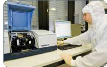
High precision measurement equipment: FTIR Spectrometer
