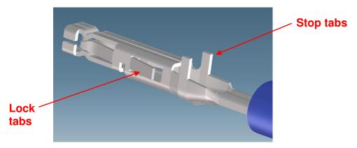
Ensure terminals are fully seated and locked during terminal insertion to the receptacle housing
