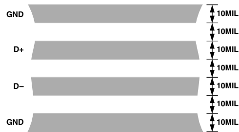
Figure 13. Arrangement of Signal Tracks
