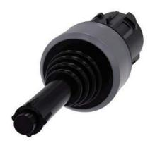
Coordinate switch, 22 mm, round, plastic with metal front ring, black, 2 switch positions, horizontal, momentary contact type, with mechanical interlocking, with laser labeling, upper case and lower case, always upper case at beginning of line
