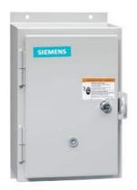
Non-reversing motor starter, Size 1, Three phase full voltage, Solid-state overload relay, OLRelay amp range 0.25-1a, 550/575 600 50/60HZ coil, Non-combination type, Enclosure type 12, Dust/drip proof for indoors, Extra-wide enclosure
