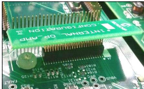
FIGURE 2: INTERNAL OP AMP CONFIGURATION BOARD
