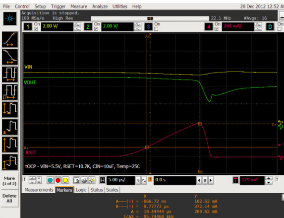
Figure 5. t_{OCp} Response Time
