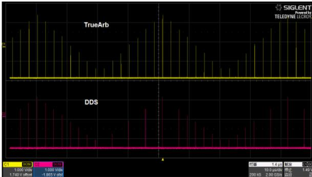
TrueArb generates arbitrary waveforms point by point, never skips any point so that it can reconstruct all the details of the waveform as defined.
