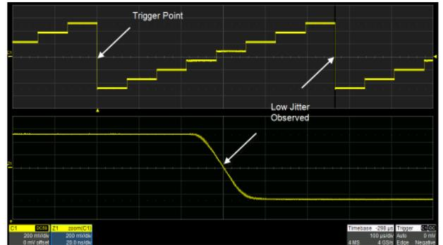
As with EasyPulse, TrueArb effectively overcomes the defect that DDS may cause the one-clock-jitter in arbitrary waveforms.
