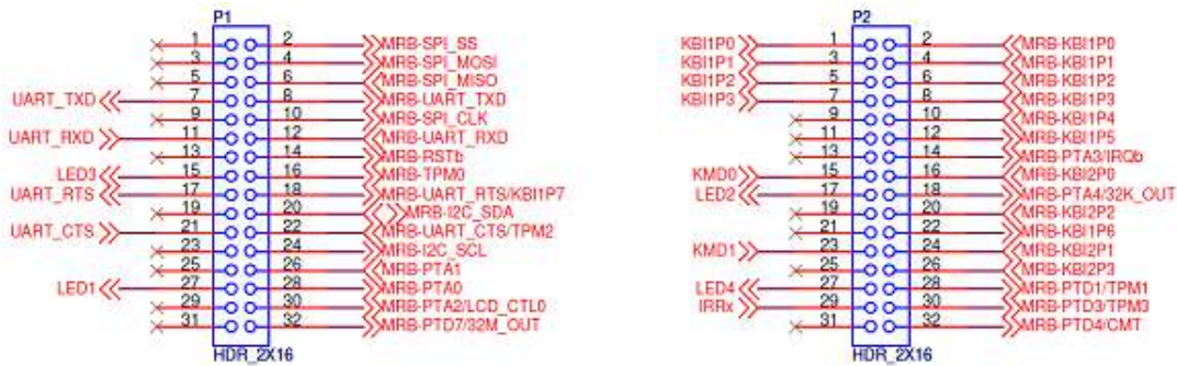
Figure 5-5. 1323x-REM IO Connector J8 and J9 Pin Mapping
