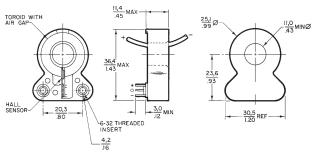
\* Application consideration: The output is clamped at the high end. Clamping voltage may be as low as 9VDC. The output will not exceed the clamping voltage regardless of field strength or supply voltage.
