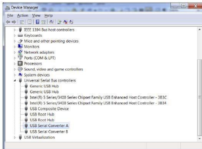
Figure A.9. Installation Completed
