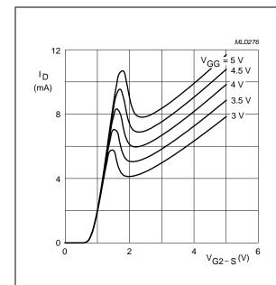
$V_{DS} = 5 \text{ V}; T_j = 25 \text{ }^{\circ}\text{C}.$
