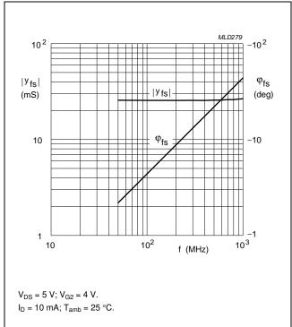
Fig.17 Forward transfer admittance and phase as a function of frequency; typical values.
