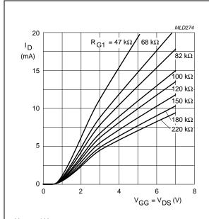
$V_{G2\text{-}S} = 4 \text{ V}.$   $R_{G1} \text{ connected to } V_{GG}; T_j = 25 \text{ °C}.$
