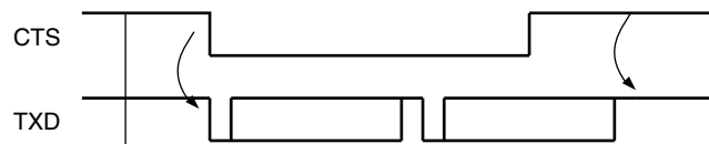
Figure 20-17. Transmitter Behavior when Operating with Hardware Handshaking
