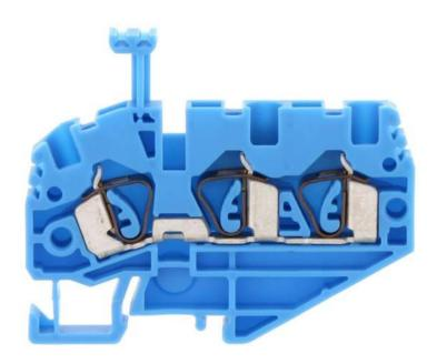
Feed-through terminal, Tension-spring connection, Mounting type: Mounting rail TS 15/5.5, Rated cross-section: 2.5 mm², Width: 5.1 mm, Colour: Blue
