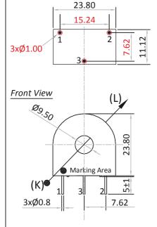
All dimensions are in mm Linear dimensional tolerance ±0.2mm
