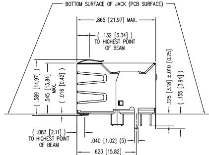
1. CONNECTOR MATERIALS: HOUSING: THERMOPLASTIC UL94 V-0 CONTACTS/SHIELD: COPPER ALLOY SHIELD PLATING: NICKEL CONTACT PLATING: SELECTIVE GOLD IN CONTACT AREA
