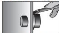
The holder will be secured at the back by two screws or nut.
