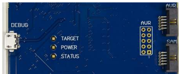
Figure 6-9. VOUT LED, used to Indicate the Status of the Target Voltage Supply
