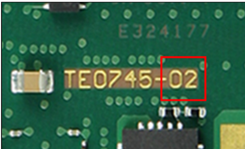
Figure 7: TE0745 module revision number.
