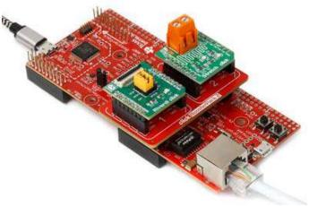
**Click BoosterPack 2** is an extension for Texas Instruments LaunchPads<sup>TM</sup> with the current BoosterPack Pinout Standard. It has two mikroBUS<sup>TM</sup> sockets onboard, for simple and easy integration of **MikroElektronika click boards** with a LaunchPad<sup>TM</sup>.
