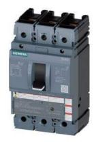
circuit breaker 3VA5 UL frame 250 breaking capacity class C 100kA @ 480 V 3-pole, line protection TM210, FTFM, In=90A overload protection Ir=90A fixed short-circuit protection Ii=10 x In nut keeper kit on both sides
