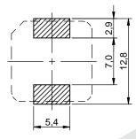
no sensitive traces underneath the component
