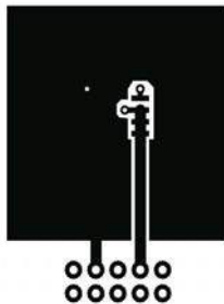
a) 50\text{ }^\circ\text{C/W} when mounted on a 1\text{ in}^2 pad of 2 oz copper.
