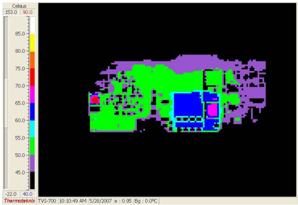
Figure 7. Thermal Map, Backside at 18Vin and 4.2Aout (Ta = 25 degrees C)
