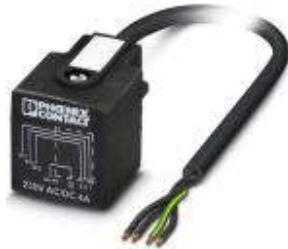
Sensor/Actuator cable, 4-position, PVC, Black RAL 9005, Free cable end, on AD valve plug (pressure switch), Cable length: 2 m
