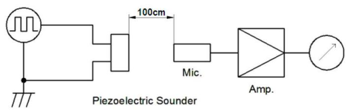
MIC: ND10 Sound Meter or equivalent Signal Generator: DF1641D or equivalent
