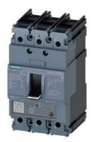
circuit breaker 3VA5 UL frame 125 breaking capacity class M 35kA @ 480 V 3-pole, line protection TM230, FTAM, In=15A overload protection Ir=15A fixed short-circuit protection Ii=10...20 x In nut keeper kit on both sides
