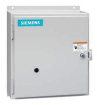
Mechanically held lighting contactor, Contactor amp rating 60Amp 0NC - 10NO poles, 208VAC 60HZ coil, Non-combination type, Enclosure NEMA type 1, Indoor general purpose use
