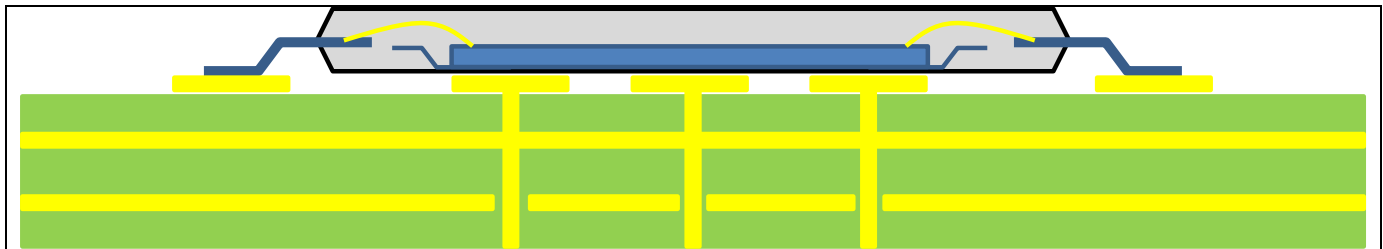
Figure 8-1: Example Thermal Via Holes on PCB.
