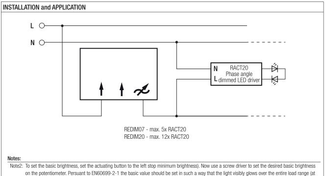
on the potentiometer. Persuant to EN60699-2-1 the basic value should be set in such a way that the light visibly glows over the entire load range (at nominal voltage -10%) when it's set to dark position.
