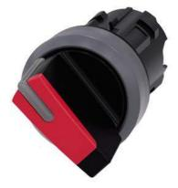
Selector switch, illuminable, 22 mm, round, plastic with metal front ring, red, selector switch, short, 2 switch positions O<I, momentary contact type, Actuating angle 45°, 10:30h/12h, with laser labeling, upper case and lower case, always upper case at the beginning of the word
