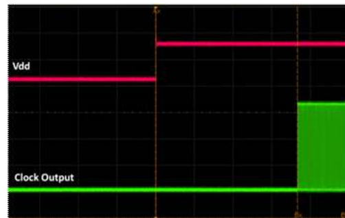
Figure 17. Startup Waveform vs. Vdd
