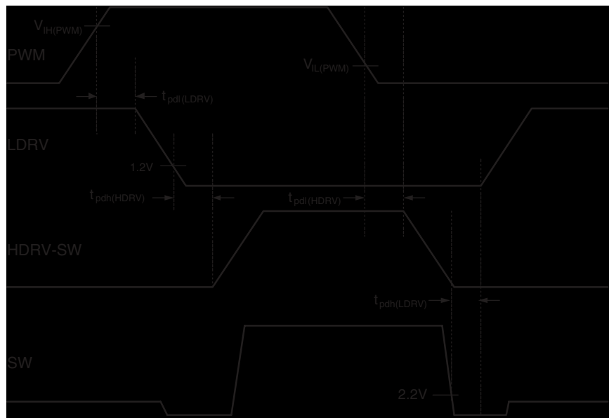
Figure 4. Adaptive Gate Drive Timing
