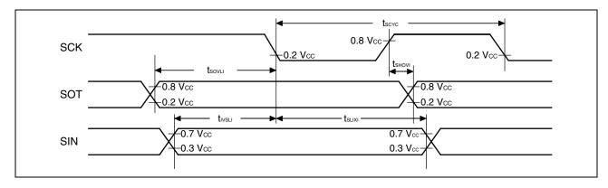
Sampling is executed at the falling edge of the sampling clock\*<sup>1</sup>, and serial clock delay is enabled\*<sup>2</sup>. (ESCR register : SCES bit = 1, ECCR register : SCDE bit = 1)
