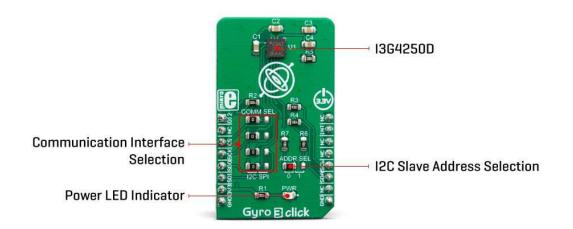
Typically, higher dps range results in lower sensitivity. Therefore, the I3G4250 allows to dynamically select the full-scale range (FSR) value in several discrete steps: ±245, ±500, and ±2000 dps. This allows optimized performance for a given usage scenario. For example, if used in applications with faster angle rates such as sports equipment monitoring (golf club or tennis racket), a higher FSR might be required, at a cost of lower sensitivity.
