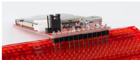
Pins soldered onto the imp Breakout Board
