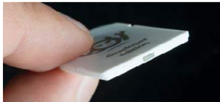
The light sensor is just behind the translucent window on the edge of the imp card.
