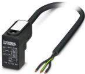
Sensor/Actuator cable, 3-position, PVC, Black RAL 9005, Free cable end, on CI valve plug (9.4 mm), with 1 LED, connected with Z diode, Cable length: 10 m
