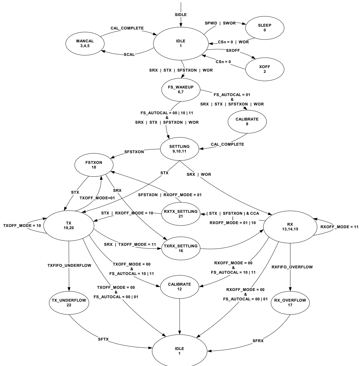
Figure 3-15. Complete Radio-Control State Diagram
